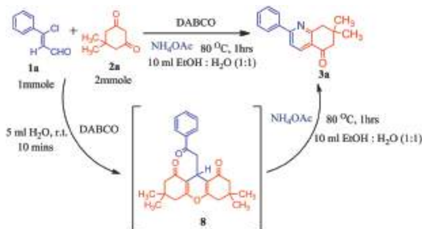
Fig. 4 Schematic diagram of the formation of dihydro-6H-quinoline-5-one derivative through xanthene-dione intermediate.
